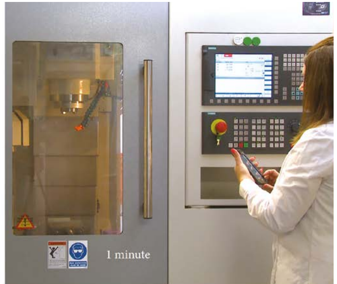
Figure 14b: Shows clearance of the smoke within a minute. Note, clearance times will differ depending on the size of the enclosure and the effectiveness of the LEV.
