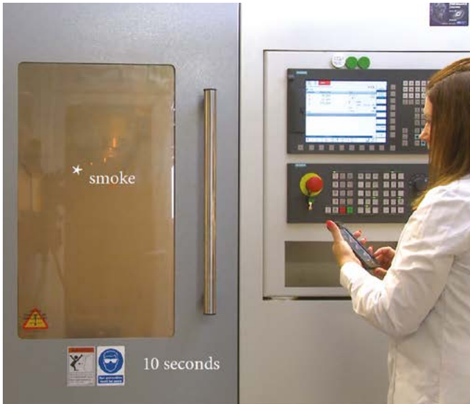
Figure 14a: Back-lit photograph of smoke generated inside a machine enclosure after 10 seconds.
